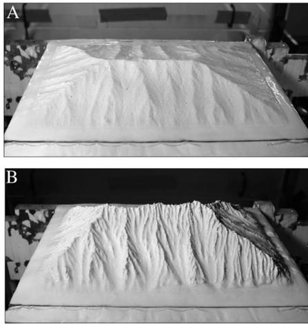
**Figure 3.** Oblique views of experiment TC18 (cf. Fig. 2). A:  $t = 240$  min. B:  $t = 480$  min. Topographies are at steady state with uplift rate of 1.5 cm/h and under high rainfall rate conditions (top: mean rainfall rate  $166 \pm 5$  mm/h) and low rainfall rate conditions (bottom: mean rainfall rate  $98 \pm 7$  mm/h).
