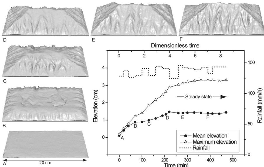
**Figure 1.** Evolution of mean and maximum elevation of experiment TC22 up to steady state, calculated from high-resolution digital elevation models (DEMs) taken at different time intervals (pixel size 1 mm). Uplift rate is 1.5 cm/h and mean rainfall rate is  $137 \pm 7$  mm/h. A–F are three-dimensional views of DEMs (A–D: growth phase; E–F: steady state). Statistical steady state is defined by constant elevation.
